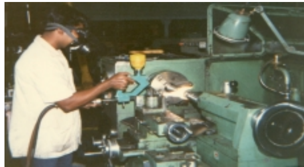
Fig.6. The thermal spraying using Rototec torch on to a circular job mounted on the lathe and rotated at optimized speed. Note the protective equipments used by the operator.
